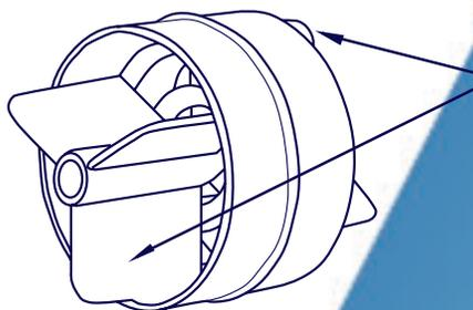
Three fins on both sides of the disc extend fully to engage with adjacent fins, thereby creating a solid wave-retention barrier. No water gets through.
