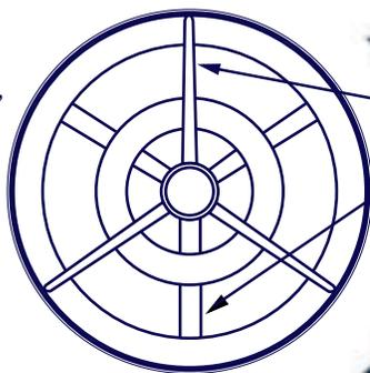
Internal ribs and walls are designed to optimize the impact-reducing capabilities of the disc, while keeping weight to the requisite level.
